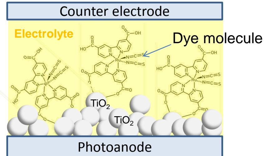
The ionized dye is regenerated by the electrolyte by a redox process where iodide is oxidized and triiodide is formed.
